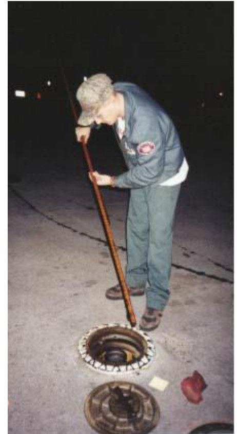
Measuring the amount of fuel in a tank
